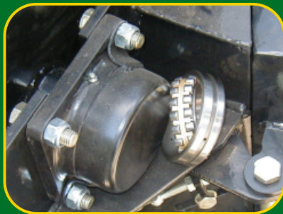
(LC900 bearing housing with exposed bearing)
